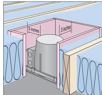
Attic rulers are required for loose-fill insulation and are a helpful guide to ensure adequate coverage. Create dams to hold back insulation and to maintain levels. Attic access such as scuttles and drop-down stairs benefit from a insulated cover.
