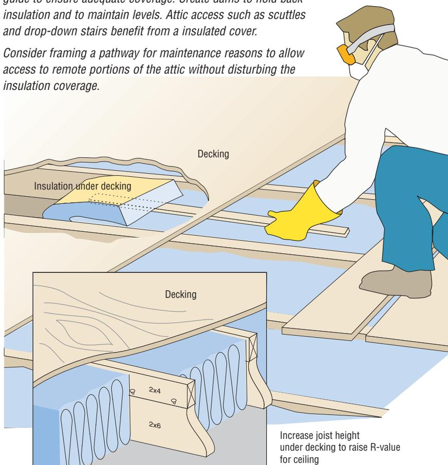
Installing insulation under existing attic decking requires some improvising to avoid removing the decking. Be sure to wear proper protective gear and clothing when installing any insulation. Install batt insulation with the vapor barrier down in attics with no insulation. If adding insulation on top of existing insulation, use batts without a vapor barrier backing or remove the backing.
